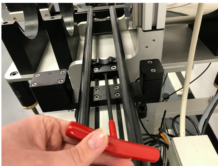
Figure 3.2: Rail sleeper removal bolt
