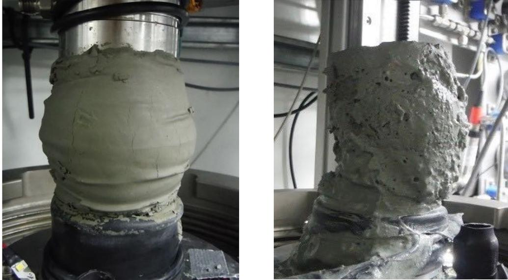
Figure 11: Samples XH-06B-7A-3 and SC-W01B-15A-5 after recovery from PCATS Triaxial. The barrel-type deformation shown by the former sample on the left is indicative of plastic deformation and strain hardening, while the clearly visible shear plane of the latter (right) indicates sudden failure typical to a brittle soil. The vesicles in the image on the right indicate ongoing degassing after recovery of SC-W01B-15A-5.
