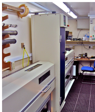
X-ray CT machine installed into 20 ft laboratory
