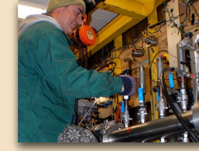
Interior view of PCATS control laboratory. Main body of PCATS is insulated. Pressure, temperature, & motion control visible to left & analysis systems right.
