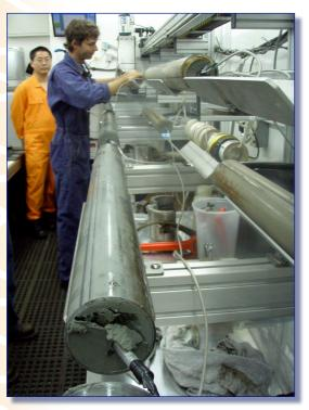
The Geotek core processing van is equipped with plenty of core racks for ease of core manipulation. Sampling and core cutting equipment, such as rotary core cutters, puncture samplers for void gas, and plug samplers for headspace gas or porewater are all available. Temperature probes are provided for direct temperature measurement if required, as well as a benchtop to wrap sections of core for storage in liquid nitrogen.
