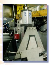
not only provides a self-preserving effect on the hydrate itself, but also cools the surrounding sediment and core liner material. Cool spots created by the unstable gas hydrate can therefore be detected on a thermal image of a fresh core that has been recovered quickly from beneath the seafloor.
