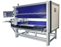
The Geotek Core Workstation (MSCL-XYZ) is a unique automated multi-core logging system for XRF, core imaging and various other surface core measurements. Multiple core sections (up to six 1.5 m core sections), or core boxes are loaded into the workstation, which are then logged in a single operation.
