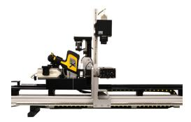
The MSCL-XZ is a benchtop or small-footprint core logging system that provides a compact solution for split core non-destructive measurements, obtaining multiple data sets simultaneously.
